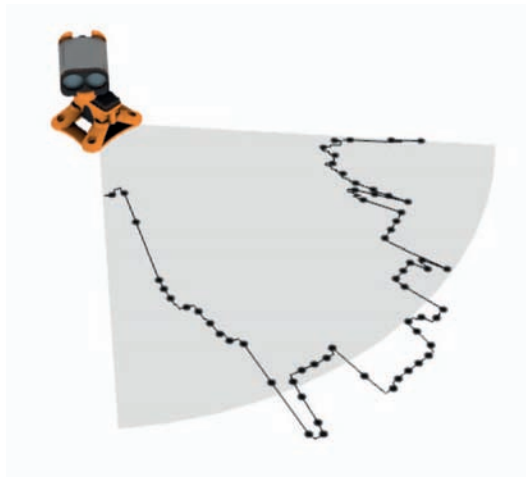
Figure 21 :: Uni-directional scanning for higher precision
